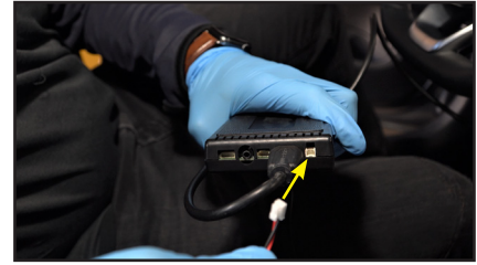
24. Plug the 2 pin power wire connector to the Smart-Play module.
