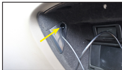
29. Run the 3.5mm plug cable towards the radio. We suggest inserting it into the hole as pictured above.
