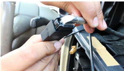
19. Plug the OEM LVDS connector to the LVDS cable provided in the kit.
