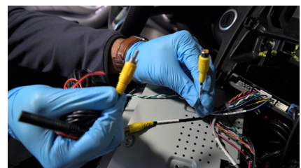
21. Install the front and rear cameras (if applicable) and power using the power wires provided.
