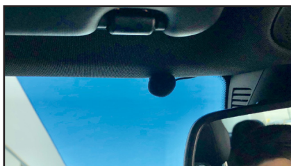
31. Mount the microphone to the desired location. Run the cable towards the Smart-Play module location and plug it into the Mic port.
