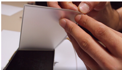
13. Gently peel off the touch panel's protective film on both sides.
