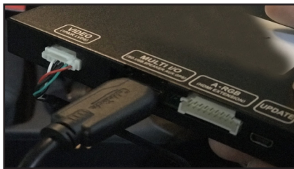
25. Plug in the 4K HDMI cable to the ACPAD-01 module.
