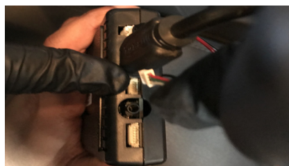
20. Plug in the other end of the touch panel PCB/cable to the Smart-Play module port next to the HDMI port.
