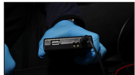
30. Plug the 3.5mm Audio plug to the Aux input of the Smart-Play module.
