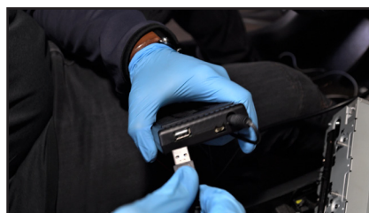
26. Plug in the USB extension cable to the Smart-Play module.
