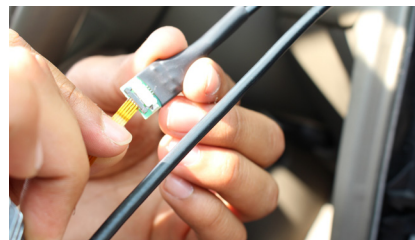
17. Connect the touch screen's flexible circuit to the touch panel PCB/cable provided.
