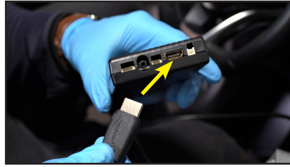
23. Plug in the 4K HDMI cable provided with the kit to the Smart-Play module.
