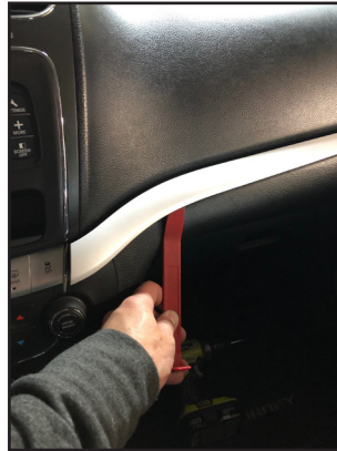
1. Use a panel removal tool to remove the left and right side trims.
