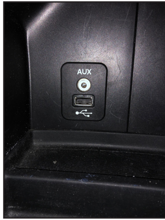
Plug the 3.5mm Aux cable to the factory Aux input.
