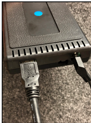
12. Plug in the USB extension cable and mic to the Smart-Play module. Run the USB extension cable to an accessible location. Run the mic cable to the A pillar.
