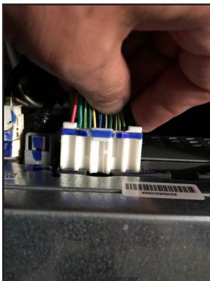
6. Unplug the radio connector and plug it to the T-harness. Plug the other end of the t-harness to the radio.
