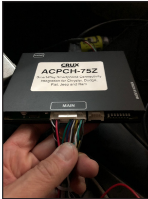
8. Plug in the main harness to the ACPCH-01 module.
