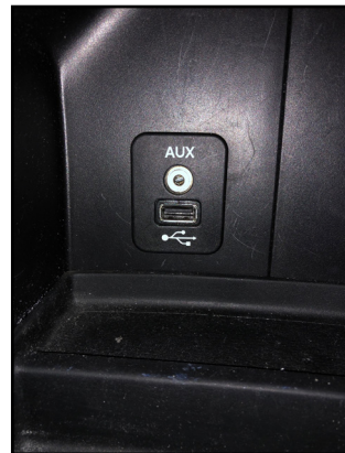
13. Plug in the Aux cable to the factory Aux input port. Possible location of this port is in the center console.
