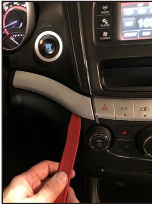
1. Use a panel removal tool to remove the left and right side trims.
