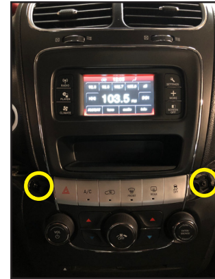
2. Remove the 2 T20 torx screws.
