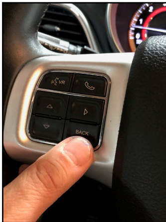
On the steering wheel controls: Press and hold the BACK button for 3 seconds.
