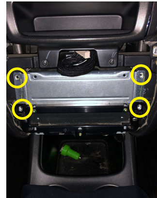
5. Remove the 4 T20 screws.
