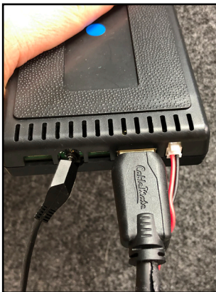
11. Plug in the power plug, 4K HDMI cable and the 3.5mm Aux cable to the Smart-Play module. Run the 3.5mm Aux cable to the factory Aux input location
