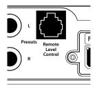
When connected to the amplifier, the HD-RLC operates as follows. At full counter-clockwise rotation, the audio will mute completely. At full clockwise rotation the level will be the same as if the HD-RLC was not connected at all. In other words, it operates strictly as a level attenuator.
