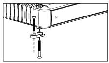
Lateral Mounting Feet are also included with your MHD600/4 to provide an alternative mounting option. Each mounting foot should be attached to the bottom of the amplifier by screwing the provided bolt into the bottom of the amplifier and up into the corner cap with the supplied 1/8-inch hex wrench. Next, using appropriate mounting screws (not included), secure the amplifier by its four Lateral Mounting Feet.
