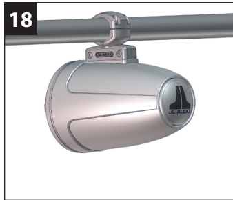
Align the aluminum logo cap to the desired angle of rotation, and press it onto the back of the enclosure. Apply masking tape (not included) to hold the cap in place until the silicone cures (at least 24 hours).
