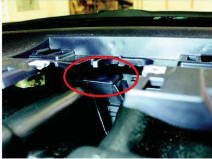
Attach the included metal plate to the interior of the vehicle's dashboard using the supplied double-sided tape.
