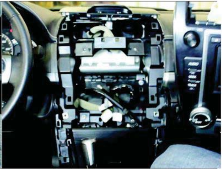
Lift screen away from dashboard.
