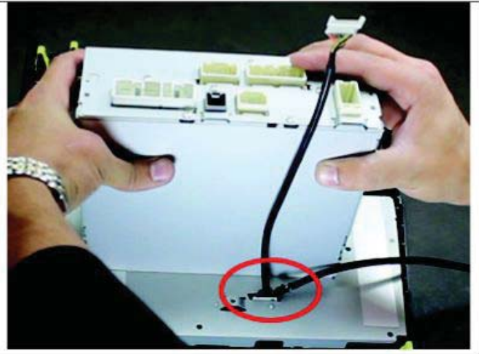
Route the LCD-IN/TP-IN Extension Harness from the radio's interior through the opening in the back of the housing.
