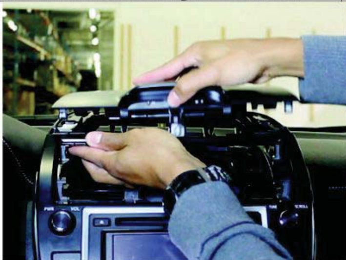
Remove upper dash trim from radio.
