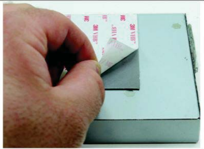
Peel the protective layer from the VHB tape making sure no debris comes into contact.
