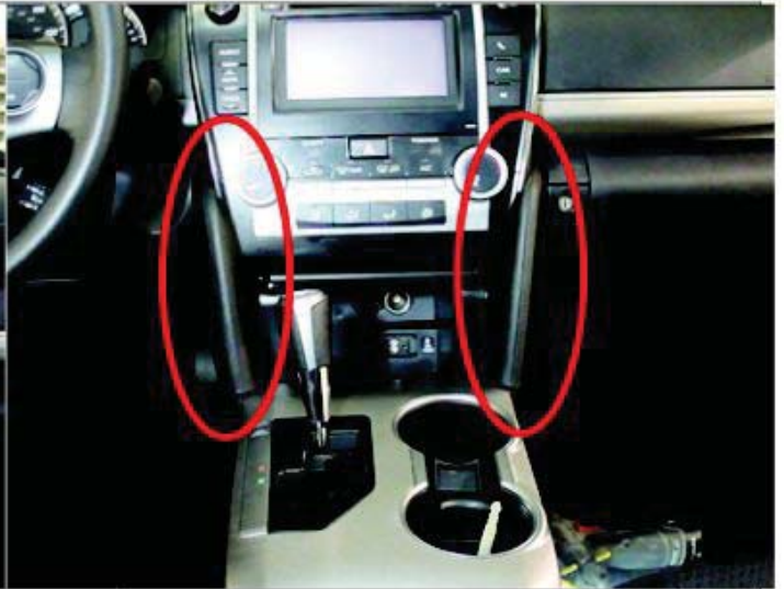
Remove trim pieces to access lower screws.
