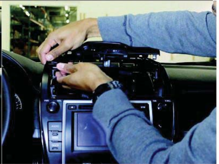
Release connectors from upper dash trim.
