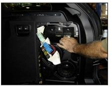
**S T E P 5 If equipped with the factory woofer system.**With a 6mm Allen key, remove the bolt that secures the top of the factory woofer enclosure.
