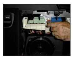
**S T E P 4**With a 7mm socket, remove the five bolts that secure the factory fuse/relay box.
