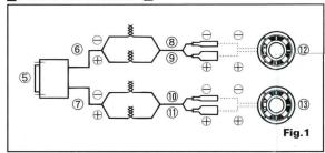
**WIRING CONNECTION (Fig. 1)** Please watch for polarity.
