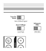
The "Low" position on the "Input Voltage" switch selects an input sensitivity range between 200mV and 2V. This means that the "Input Sens." rotary control will operate within that voltage window. If you are using an aftermarket source unit, with conventional preamp level outputs, this is the position you should select.
