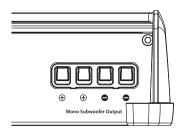
You will notice that there are two "+" positive connections and two "-" negative connections. This is to facilitate multiple subwoofer wiring. The two positive and two negative connections are connected in parallel inside the amplifier. They are not stereo outputs. Connecting two subwoofers, each to one set of positive and negative terminals, will result in a parallel subwoofer connection. When only connecting one pair of subwoofer wires, it is not necessary to use both sets of connections.
