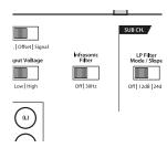
With ported enclosures, the use of the "Infrasonic Filter" is highly recommended to protect the speaker(s) from excessive excursion below box tuning.
