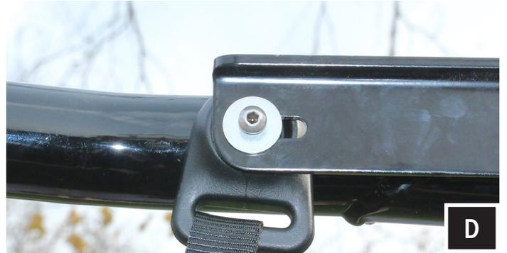
D. While holding the enclosure in position use the supplied 30mm hex bolt (1) aluminum spacer and factory washer to secure the PN304 bracket to the safety net bracket. Do not tighten it all the way. Repeat these steps on the opposing side.
