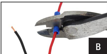
B. Crimp the supplied fuse holder onto the end of the RED wire and attach to the battery "+" terminal.
