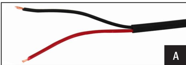
A. Cut the power/ground cable to length; be sure to leave enough wire at the battery location to wire to the battery, strip back approximately 4 inches of the black tubing to expose the red/black wires inside. Strip back 1/4"-1/2" of wire to make your connections.
