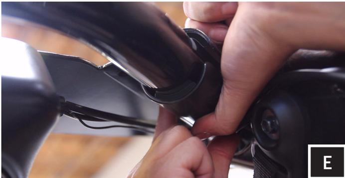
E. Install both bottom J Brackets using (4) Phillips screws (8) Washers and (4) lock nuts. Be sure rubber inserts are pre-installed.
