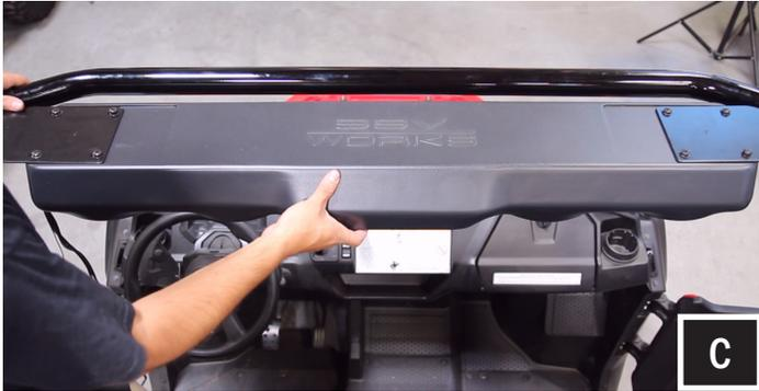
C. Place the WP3-PN304A onto the cage with the (2) J style brackets resting on the front of the cage.
