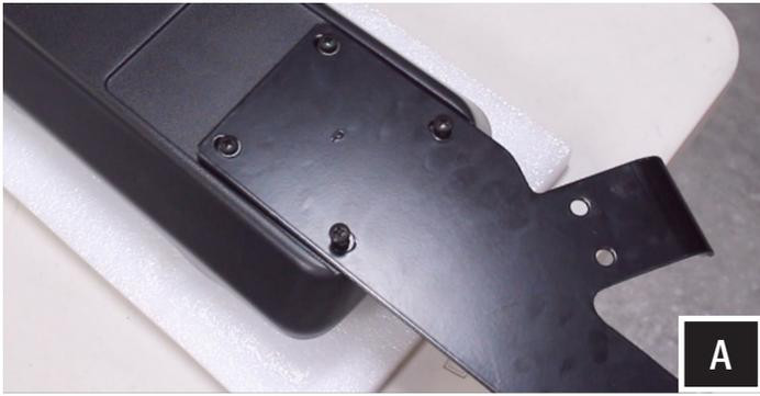
A. Loosely install the (2) mounting brackets onto the top of the enclosure using (8) Phillips Screws and (8) washers. Brackets are marked with a D (driver) or P (passenger) for correct orientation.
