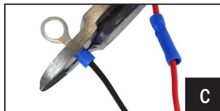
C. Crimp the supplied ring terminal to the BLACK wire and attach to the battery "-" terminal.
