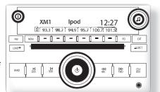
rotary knob will display AUX 1 or AUX 2. Press the **FWD>>** too select (AUX 1 = iPod no radio control and AUX 2 = Device 2). To change from Device 1 to Device 2 you will need to switch to FM or CD mode and back to XM to gain access to the mode select menu.
