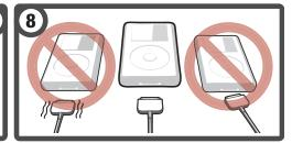
Connect iPod to GMPD2 iPod dock connector. Plug the connector in straight. Do not insert the cable at an angle or wiggle the cable during insertion.
