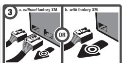
Disconnect double multi-pin factory Disconnect 16-pin factory connectors from your factory radio (see below for distrib).
