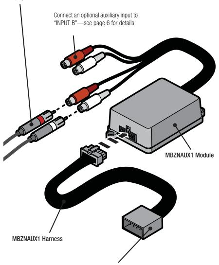
**10-pin Female Connector.** Remove the factory radio and connect the 10-pin male connector to the rear panel. Read the instructions on pages 5 and 6 for further details.
